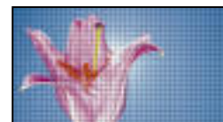
The typical 'screen door' effect seen on projectors without SXRD™ technology.
